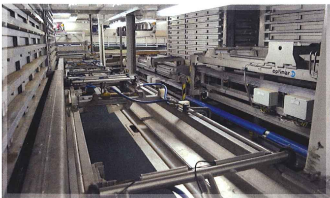
The compact factory features plate freezers that don't need to be defrosted frequently.
