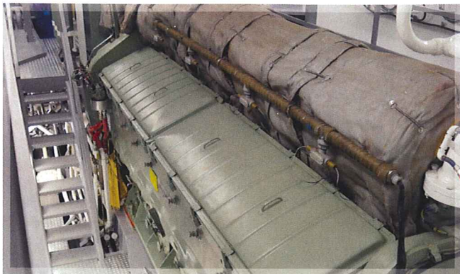
The Araho's single main engine is a 4,000-hp EMD that turns 900 rpm.
